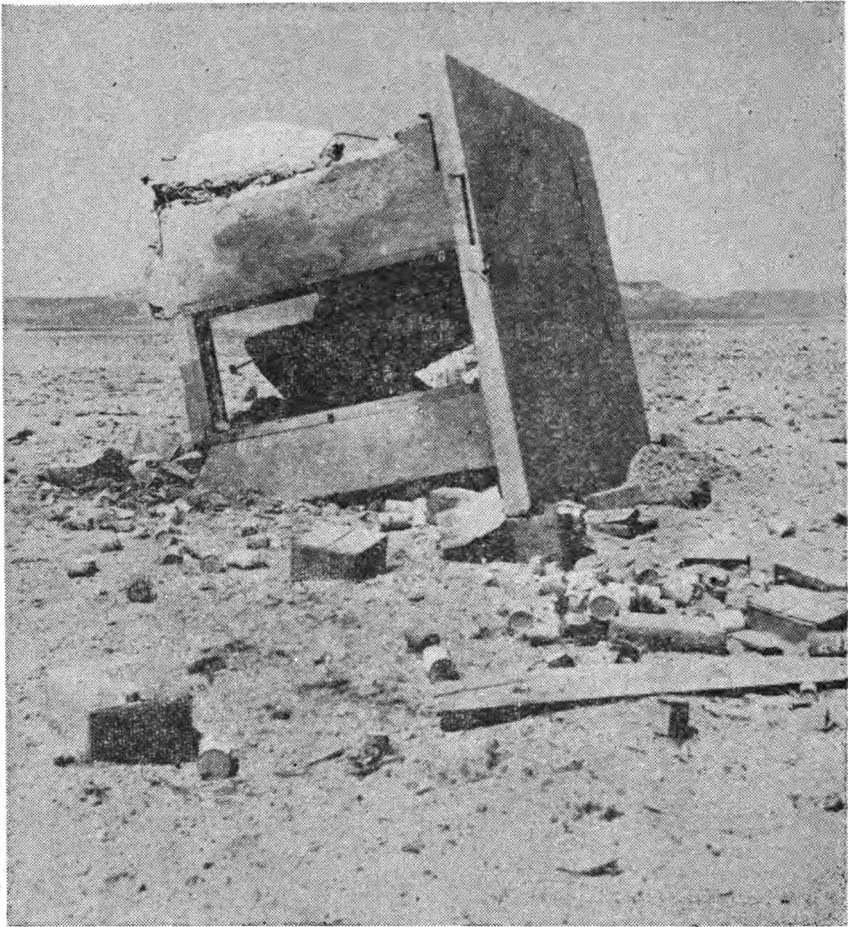
FIGURE 6.—Structure after a peak overpressure in excess of 11.6 pounds per square inch.
